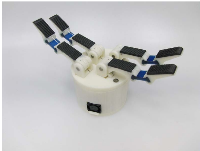
Figure 66. Sample End Effector from the Yale OpenHand Project. Source: [50].
